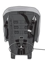
Attach the harness straps **B** to the splitter plate (i) using the *infant position* (page 37) on the harness straps. As your child grows, you can attach the harness straps
