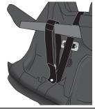
Pull until just taut and adhere Velcro to itself, as shown. (Overtightening could cause the strap to detach from the product).
