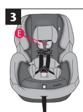
To remove the harness covers ①, follow steps for Positioning the Harness Strap (p. 36). After Step 2, slide harness covers off harness straps. Continue with Step 3.
