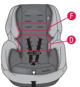
Make sure the harness straps are in one of the **three lower** strap slots **①**. The harness straps **MUST** start at shoulder height or lower, using the strap slots closest to your child's shoulders **③**, as shown.
