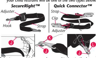
Refer to your vehicle owner's manual to locate the lower anchor bars **1** on your vehicle seat. Attach the right hook (), or clip (), to the right anchor bar () and the left hook, or clip, to the left anchor bar. DOUBLE CHECK that the lower anchor connector hook is fully engaged by pulling hard on the lower anchor connector strap.
