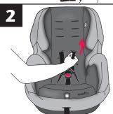
Pull harness strap through to the front of the child restraint. Thread each harness strap through the appropriate slot. Pull the harness strap to the back of the child restraint.
