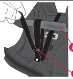
When the recline stand is in the **recline position**, wrap Velcro® strap around the recline stand (a) and insert the end of the strap through the D-ring (b), as shown.
