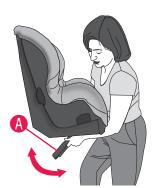
Lift the child restraint and flip the recline stand (1), located under the child restraint seat, to either the **upright** or **recline position**.
